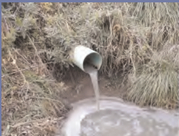
Figure 3. Contamination of subsurface drainage effluent attributable to heavy rainfall following application of liquid swine manure to an untilled, corn silage field in Darke County, Ohio. Analysis of the effluent indicated a BOD 5 of 3200 mg/L, 205 mg NH 4 -N/L, 9.0 mg NO 3 -N + NO 2 -N/L, and 174 mg total P/L. Courtesy of OEPA.
